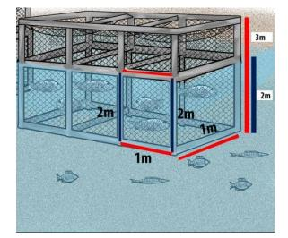
Figure 1. Schematic of the experimental device in each water reservoir.
