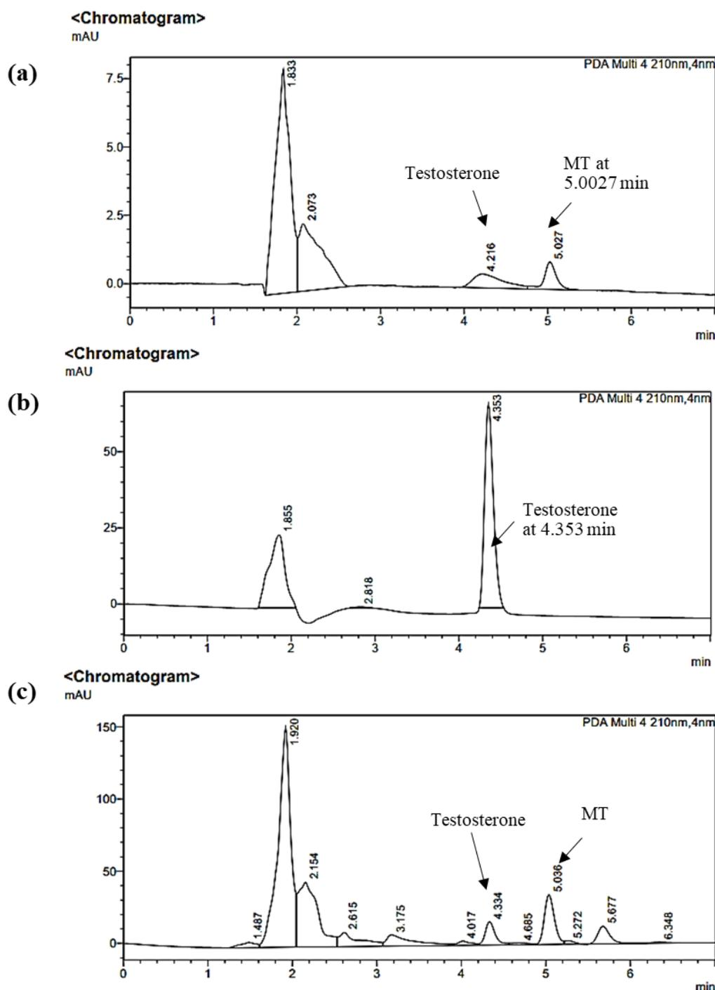
**Figure 4.** HPLC chromatograms of (a) standard solution of MT (1 mg/L) containing Testosterone (T) as an internal standard (IS) (b) T recovered spike from the IS-only solution (60 mg/L) (c) MT recovered spike of the extract from the fry of tilapia (MT at 5.0036 min; T at 4.334 min).
