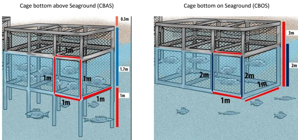
Figure 1. Schematic of the experimental device in each water reservoir.
